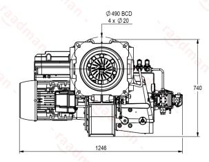
Suggested boiler flange diameter = 350 mm
